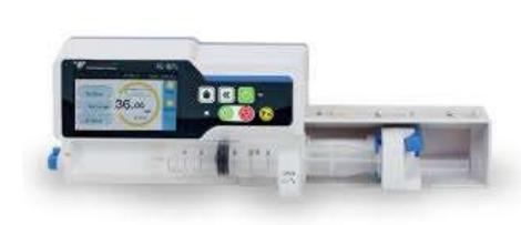
It's a small, lightweight, battery operated, portable pump, used to administer medications to the pt. slowly and steadily over a period of time, usually 24 hours.
